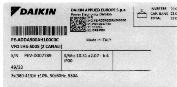
Fig. 31– VFD LHS Identification Label
