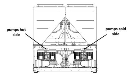
When the Inverter Kit for pump is selected the 1 inverter for each motor pump is provided.
