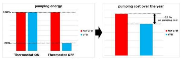
Thanks to the saving on pumping cost, the payback time for the Inverter Kit is approximately one year.
