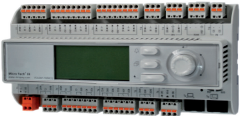
The POL638 standard software has been customised to manage the control signals of Daikin's ERQ and VRV IV systems.
