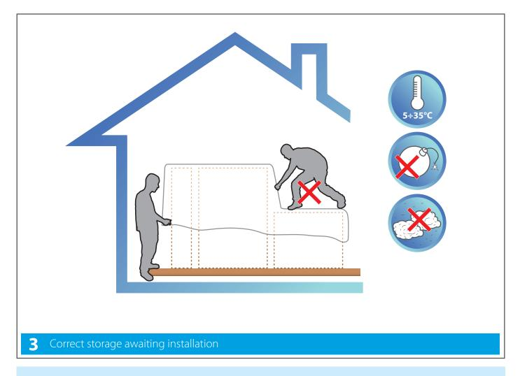
Any movement carried out after unpacking must be done with the doors closed. Do not move the units by pulling on the doors, if present, the uprights or other protruding parts that are not an integral part of the structure.
