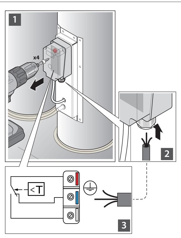
Connect to the red and blue terminal. The contact will close when the temperature drops.
