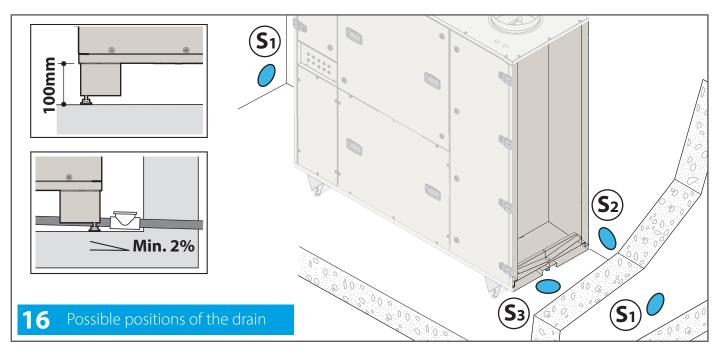
The drain pipe must have a larger diameter than the unit drain (3/4 "F) and a minimum inclination of 2% in order to guarantee its operation.
