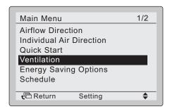
3. Press the Up/Down buttons to select the Ventilation mode and press the Menu/Enter button.
