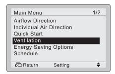
3. Press the Up/Down buttons to select the Ventilation rate and press the Menu/Enter button to confirm
