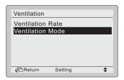
4. Press the Up/Down buttons to select the required ventilation mode. For more information on ventilation modes, see the reference guide for the installer and user.
