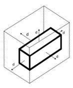
where Ad being the surface around the chiller calculated
