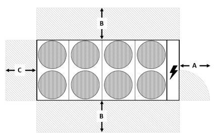
Space requirements Each side of the unit must be accessible after installation for periodic service.
