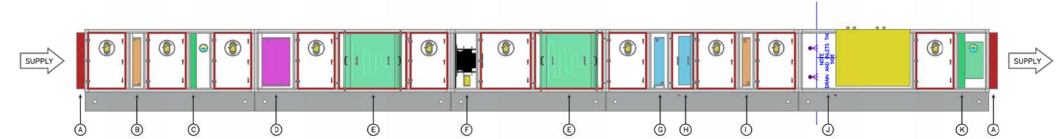
A: Minimum class 3 (BS EN 1751) Aluminium opposed blade low leakage dampers with no plastic parts, suitable for motorisation & included to all openings. Spring return actuators with end switches by others. SS304 & SS316 construction also available.
