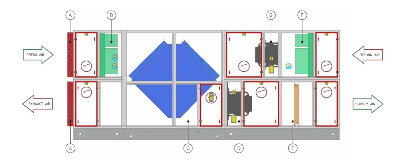
A: Class 4 aluminium epoxy coated opposed blade low leakage dampers.
